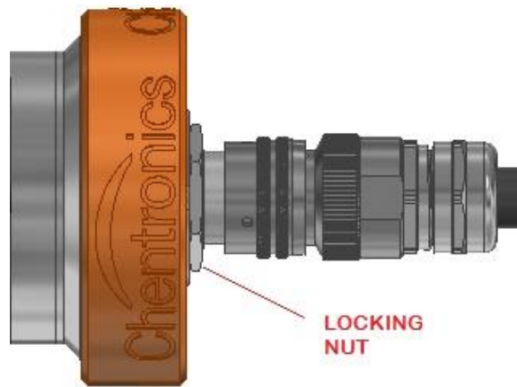
FIGURE B: SEAT THE CONNECTOR AND SEAT THE LOCKNUT AGAINST THE CONNECTOR BARREL.
